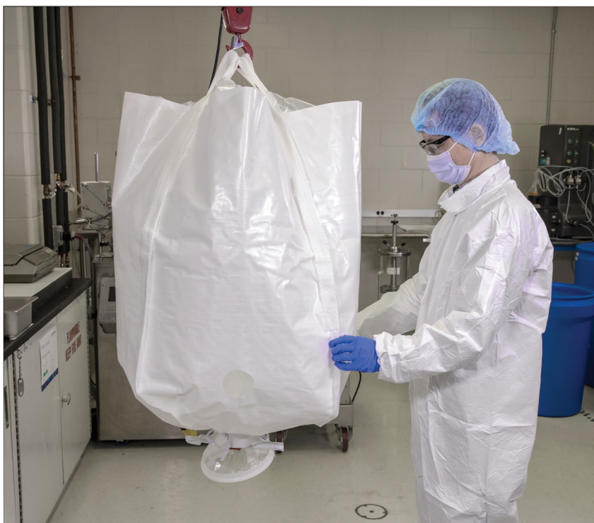
Figure 1. The use of pre-packaged materials can help address some of the challenges faced with typical powder-handling processes, such as subdividing, weighing, and dispensing.
