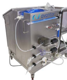
FIGURE 3: Buffer prep strategy using in-line dilution (ILD), single use systems & buffer concentrates delivered as raw materials.
