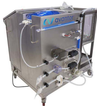
FIGURE 3: Buffer prep strategy using in-line dilution (ILD), single use systems & buffer concentrates delivered as raw materials.
